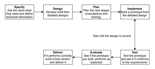
Fig 4A – The design process.
