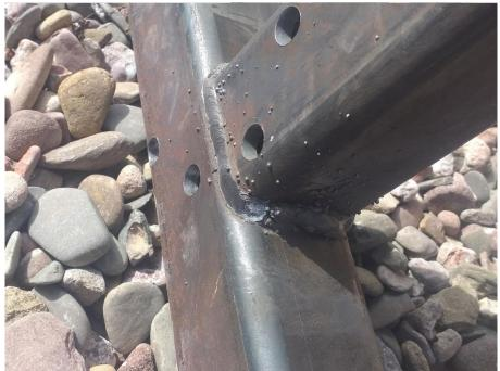
Fig 5B – An image showing a continuous weld between two lengths of box section.
