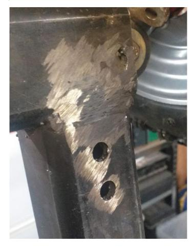
*Fig 5E – A patch of material that has been linished.*
