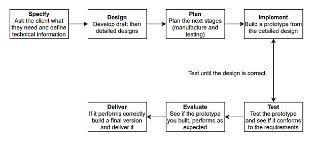
Fig 2A – The design process.
