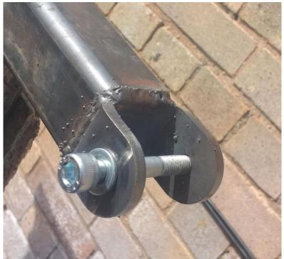
Fig 5C – An image showing the kingpins welded to the chassis box section.
