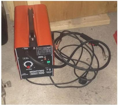
Fig 5A – Image showing the welder used in the chassis production.
